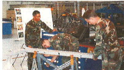
Armament Systems Technicians inspect AIM-9 Missile Launcher (Missile to Aircraft Interface)
